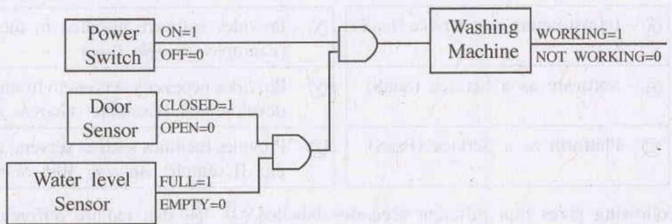
The following is the truth table equivalent to the above logic circuit. Write down labels (A) - (H) and the corresponding truth value (1,0) of each label.
